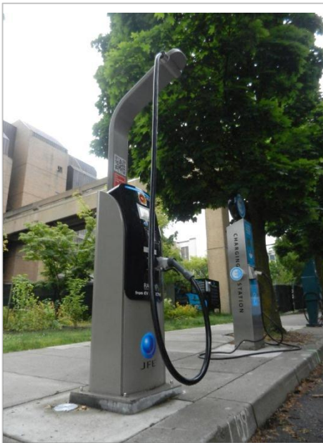
Suspending cable assists with handling
