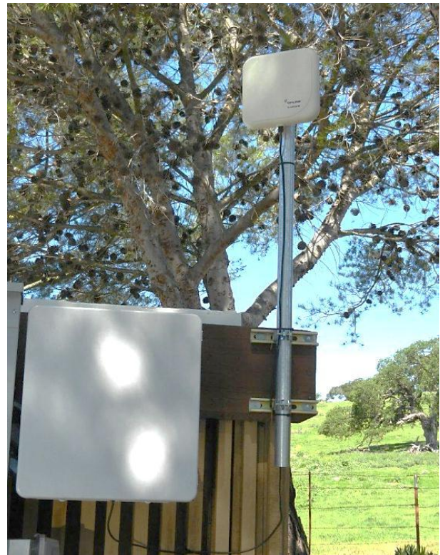
Directional antenna sends data from remote parking location
