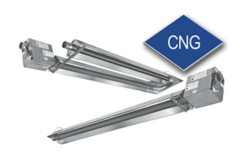
Several manufacturers now produce gas-fired radiant tube heaters with surface temperatures below 750°F. These units should be designed and recommended by the heater manufacturer for CNG garages, must be installed with a sealed and ducted combustion air source and must be monitored and controlled to keep temperatures below 750°F.
