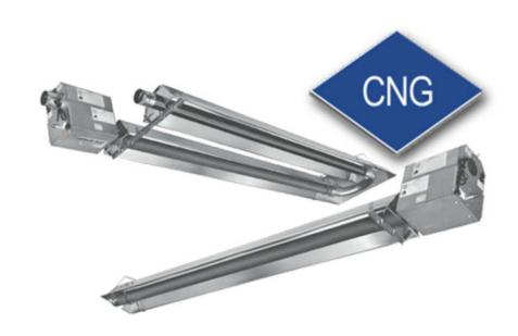
Several manufacturers now produce gas-fired radiant tube heaters with surface temperatures below 750°F. These units should be designed and recommended by the heater manufacturer for CNG garages, must be installed with a sealed and ducted combustion air source and must be monitored and controlled to keep temperatures below 750°F. Radiant heating systems that are safe for CNG are also safe for LNG.
